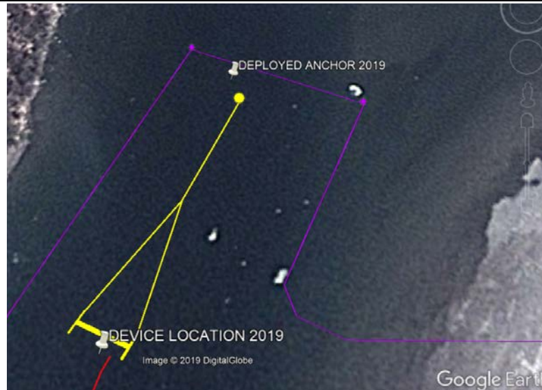
Figure 20. Measured final anchor position and estimated device position following anchor setting
