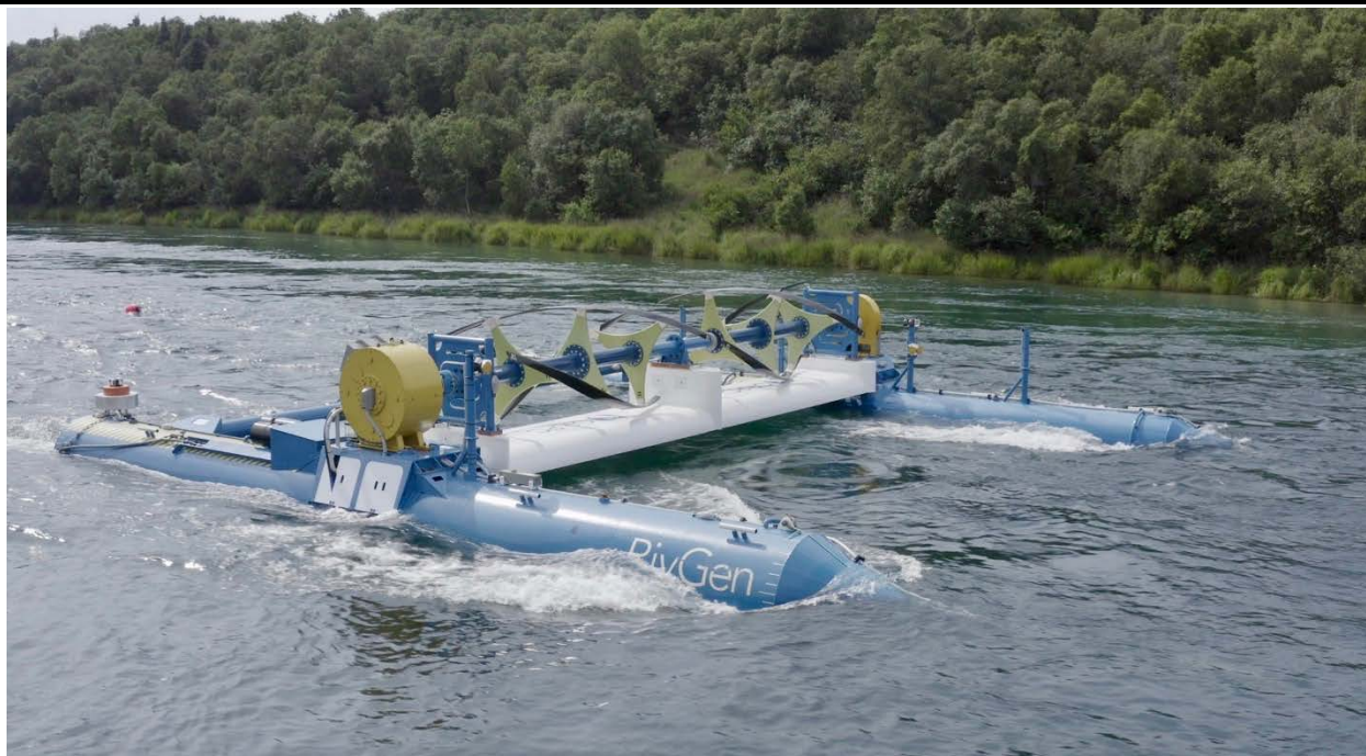
Figure 25. Installed RivGen device on its mooring system
