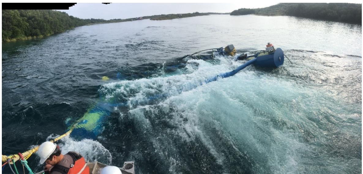
Figure 27. End pivot launch (bow down) deployment attempt
