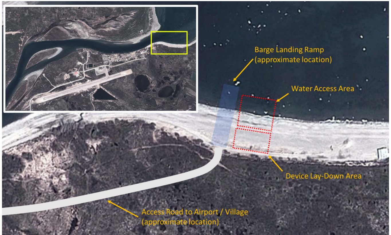
Figure 2. ORPC RivGen device assembly site, overview
