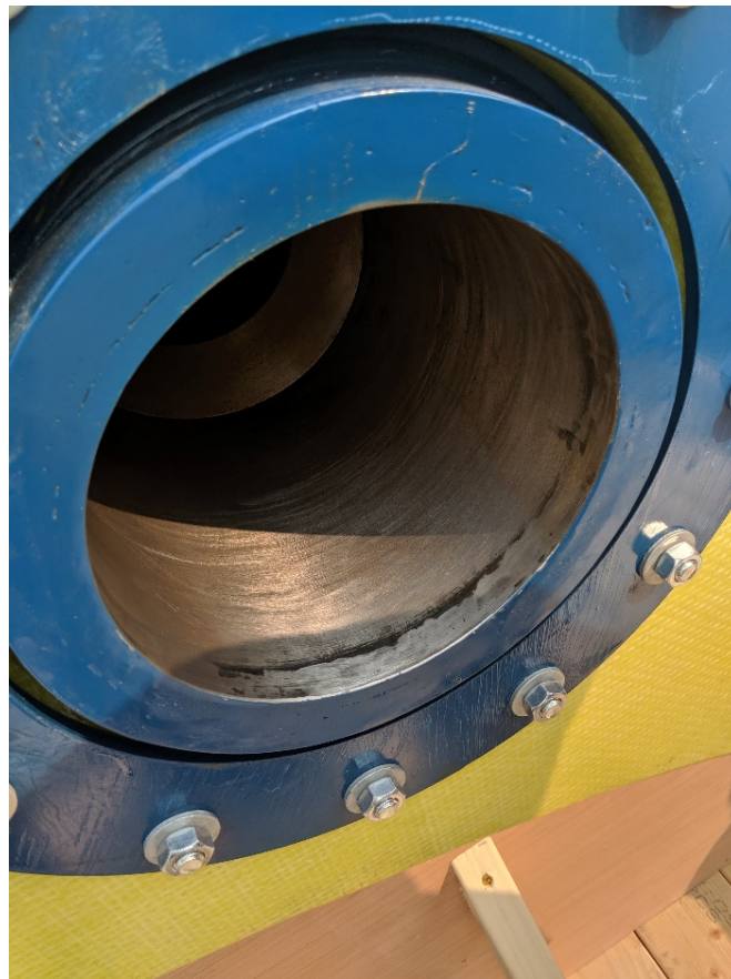
Figure 9. Example of a turbine shaft ID as received. Measurements and visual inspection indicated shaft ID did not meet fabrication specifications.
