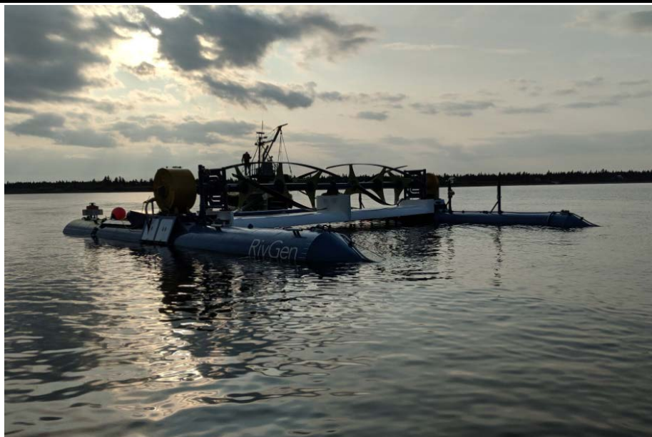
Figure 24. RivGen device following still water deployment and retrieval tests
