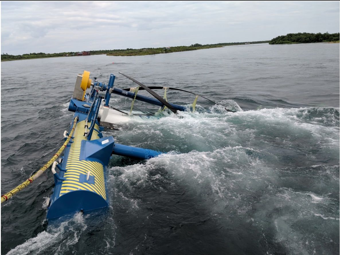
Figure 26. Side pivot launch in-river deployment test
